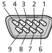
**RS-232 Serial Cable DB9 Pins (PC End)**
