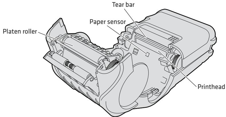
**PB22 and PB32 Mobile Label and Receipt Printer:** You need to clean these parts regularly.
